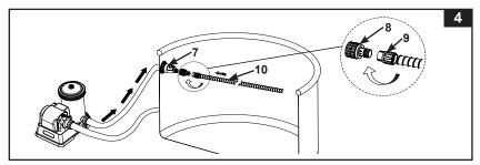
Extend the hose (10) to the furthest opposite side of the pool wall or to the furthest corner of the pool so that it overhangs the wall, and then cut the excess hose with a scissor. See Fig. 5.
